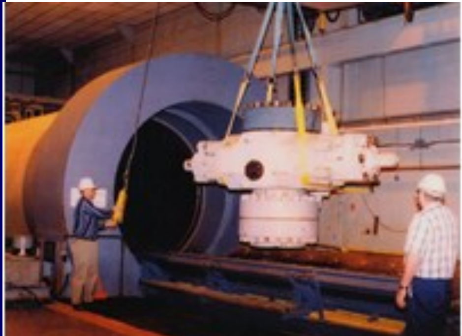
Pressure Test of Subsea Blowout Preventer Section
